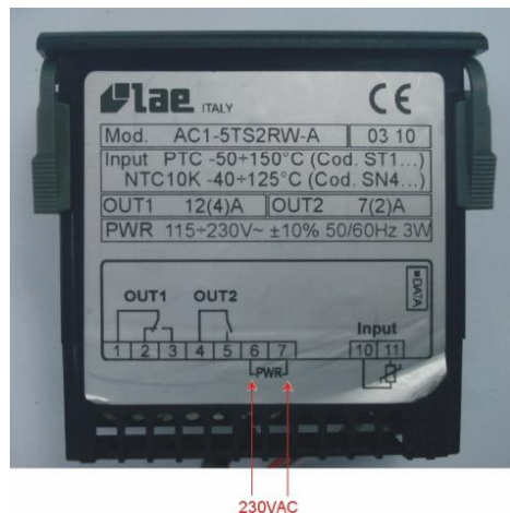
Circuit connection for new one
