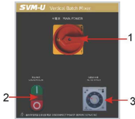
Picture 4-1: Description of Control Panel
