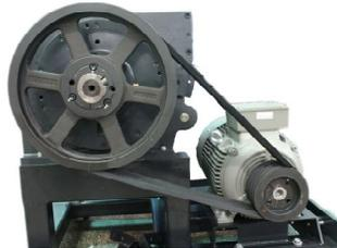
Picture 6-6: Installation of Belt Pulley and Motor 2
