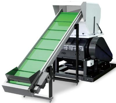
Material feeding for traditional large granulators is quite a difficult matter. They are generally installed at a lower place or a platform must be built for material feeding. Shini has particularly designed the belt conveyor to easily convey the material into the cutting chamber of SG-43 series. Add "BCF" at the end of the model code.
