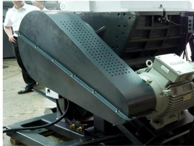
Picture 6-8: Installation of Belt Pulley and Motor 4
