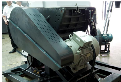
Picture 6-10: Installation of Belt Pulley and Motor 4
