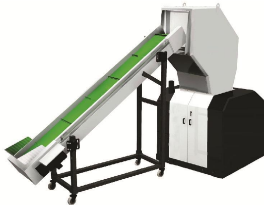
Picture 2-12: Belt Conveyor
