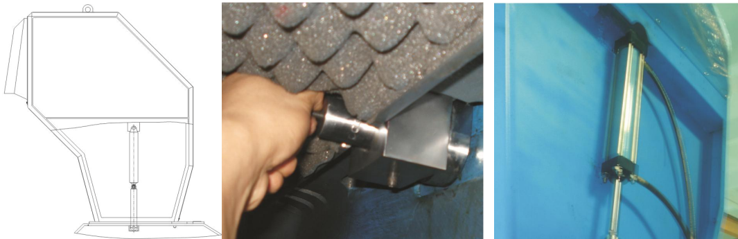
Picture 3-11: Schematic Diagram of the Feeding Box Oil Cylinder Installation
