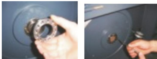
Picture 3-6: Installation of Belt and Belt Pulley 3
