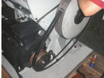
Picture 3-6: Installation of Belt and Belt Pulley 3
