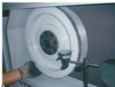
Picture 3-5: Installation of Belt and Belt Pulley 2
