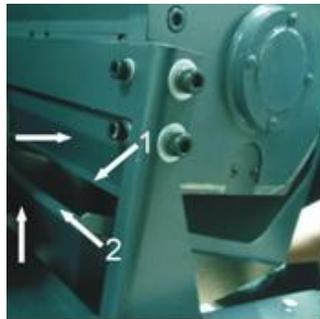
Picture 3-11: Installation of Material Storage Box 2
