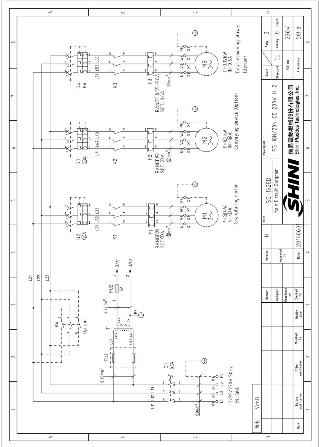
Picture 2-12: Main Circuit Dia. (230V)
