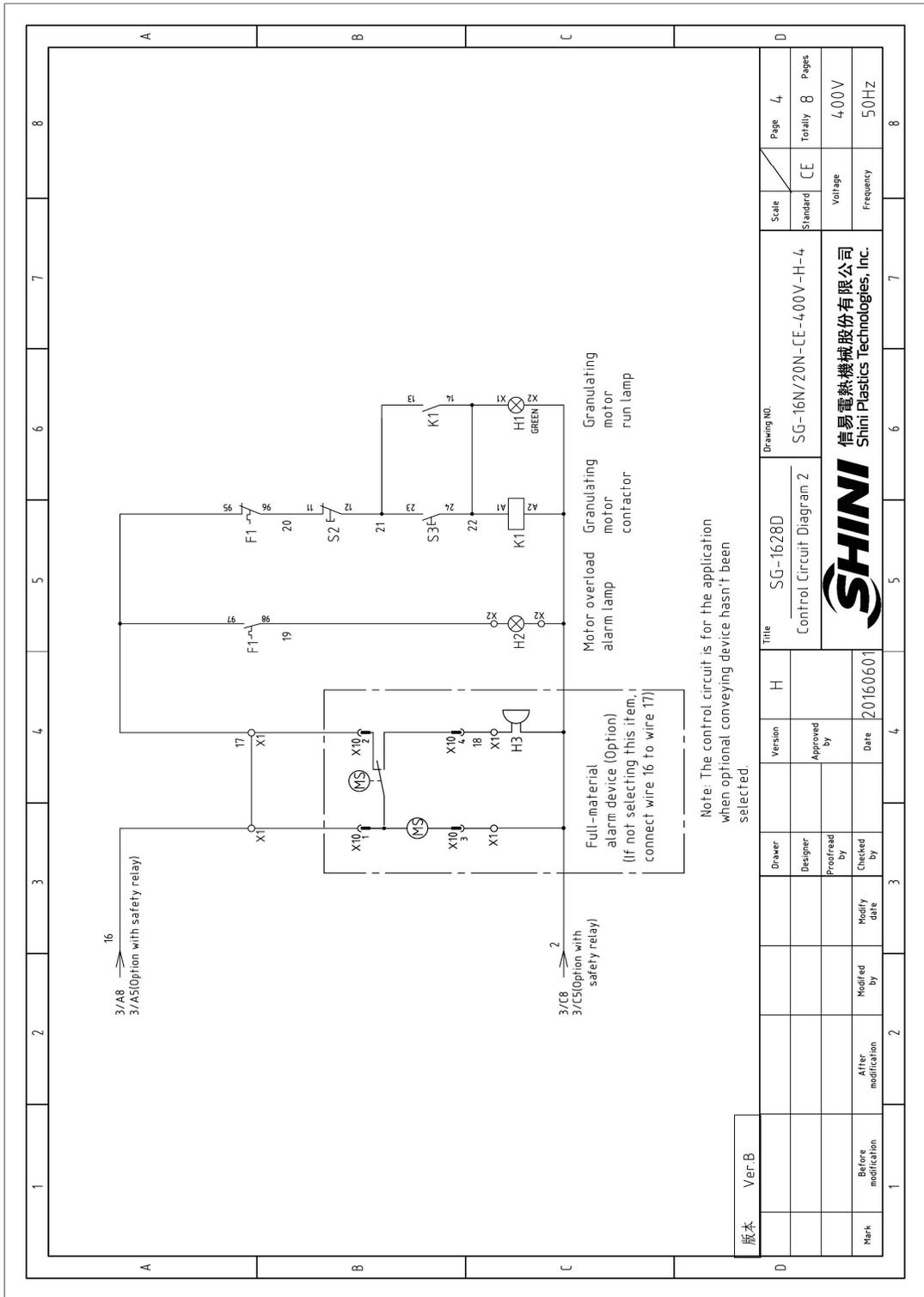
Picture 2-19: Control Circuit Dia. 2 (400V)
