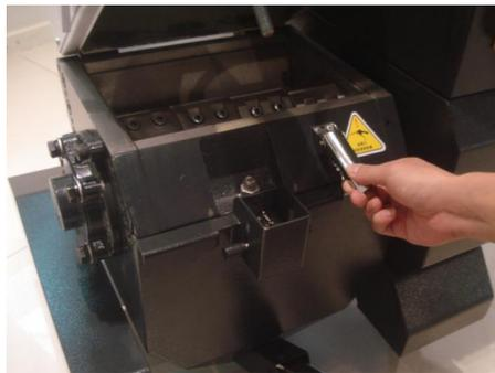
Picture 3-13: Installation of Material Storage Box 4
