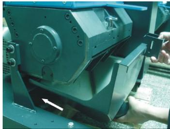
Picture 3-10: Installation of Material Storage Box 1
