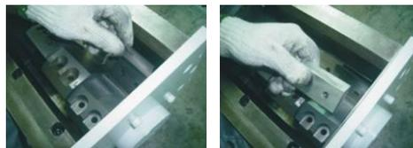
Picture 3-4: Installation of Rotating Blade and Fixed Blade 1
