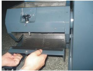
Picture 4-4: Open the Screen Bracket and Screen 2
