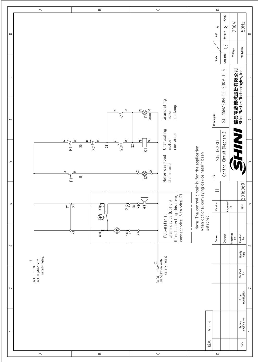
Picture 2-14: Control Circuit Dia. 2(230V)
