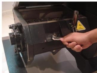
Picture 4-3: Open the Screen and Screen Bracket 1
