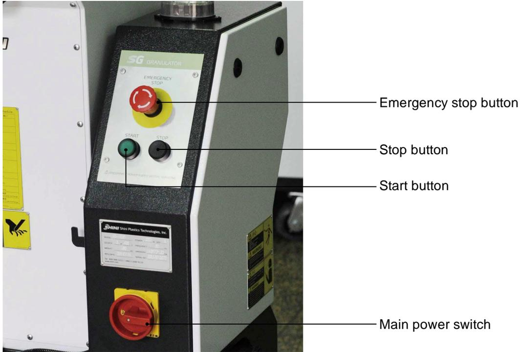
Picture 4-8: Stop, Emergency Stop and Startup button
