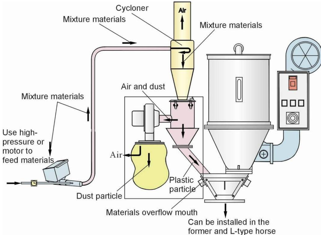
Picture 2-28: Dust Separating System materials inlet
