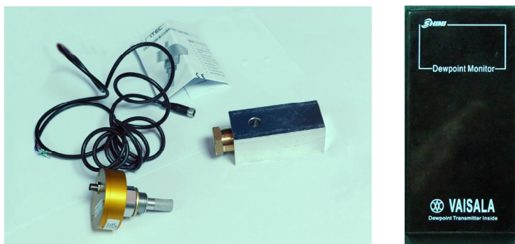
Picture 6-6: Parts of Dew-point Monitor
