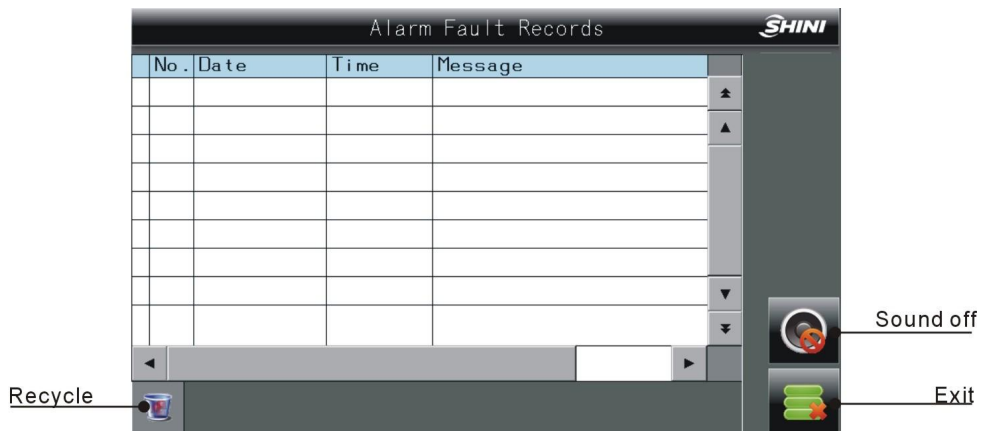
Picture 4-15: Alarm Fault Records
