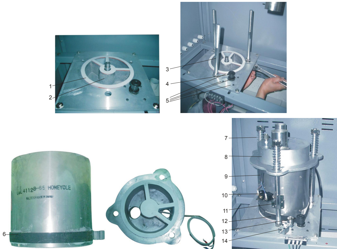
Picture 6-3: Installation of The Rotor
