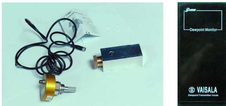
Picture 6-6: Parts of Dew-point Monitor
