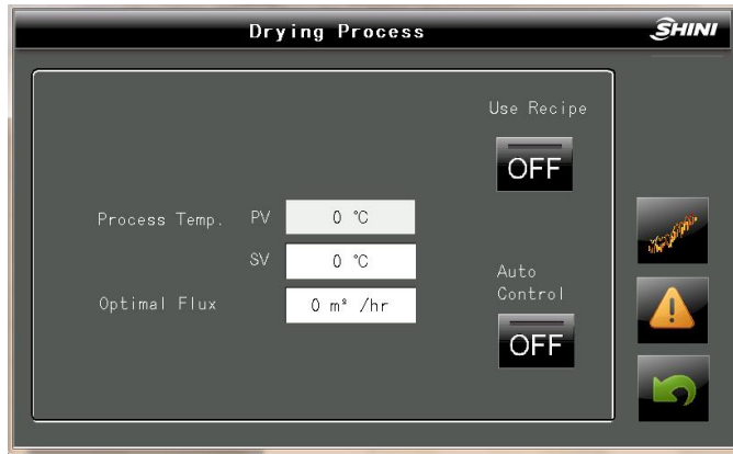
Picture 4-16: Drying Process Screen
