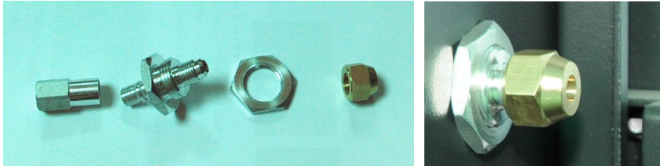
Picture 6-7: Copper Joint Assembly of Original Machine
