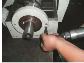
Picture 3-5: Installation of Bearing and Blade Rest 3
