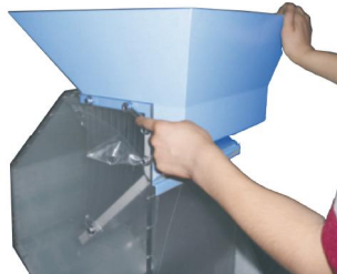
Picture 3-13: Installation of Feed Box, Feed Port and Storage Bin 3
