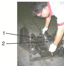
Picture 3-4: Installation of Bearing and Blade Rest 2
