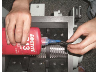
Picture 6-1: Blades Maintenance
