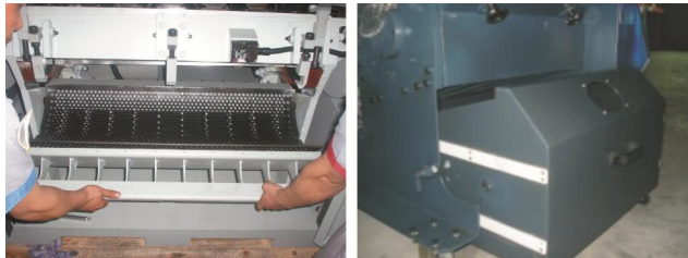
Picture 3-10: Installation of Regrind Storage Bin, Screen and Screen Bracket
