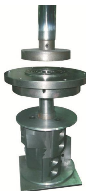
Picture 3-5: Installation of Bearing Block and Bearing
