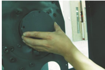
Picture 3-6: Installation of Bearing Cover
