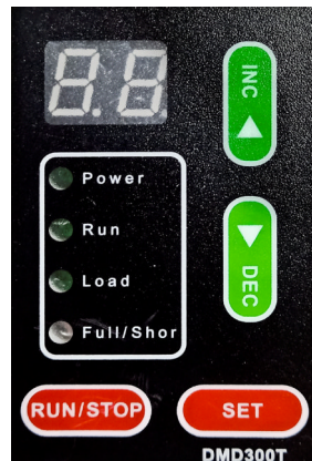
Picture 4-1: Control Panel
