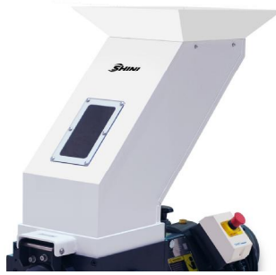
Picture 6-7: Installation of Feed Box, Feed Port and Storage Box 1
