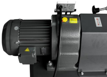
Picture 6-6: Installation of Gear Motor 3
