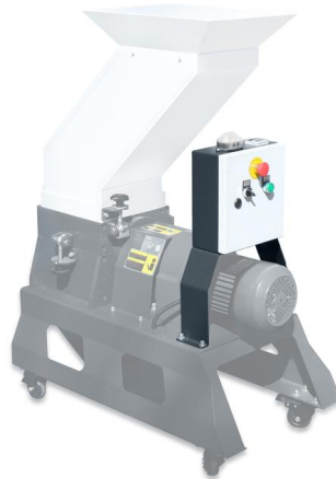
Picture 2-8: Control box with intermittent running function
