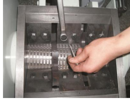
Picture 6-14: Installation of Fixed Blades and Rotating Blades 3
