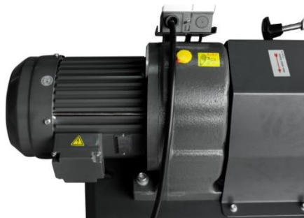
Picture 6-6: Installation of Gear Motor 3
