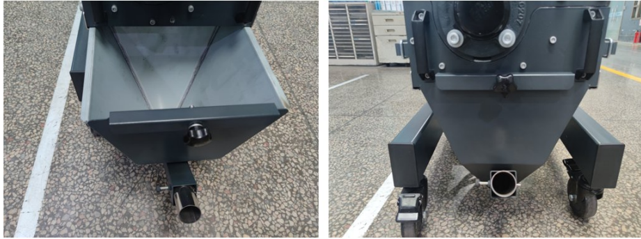
Picture 6-6:Installation of Storage Box
